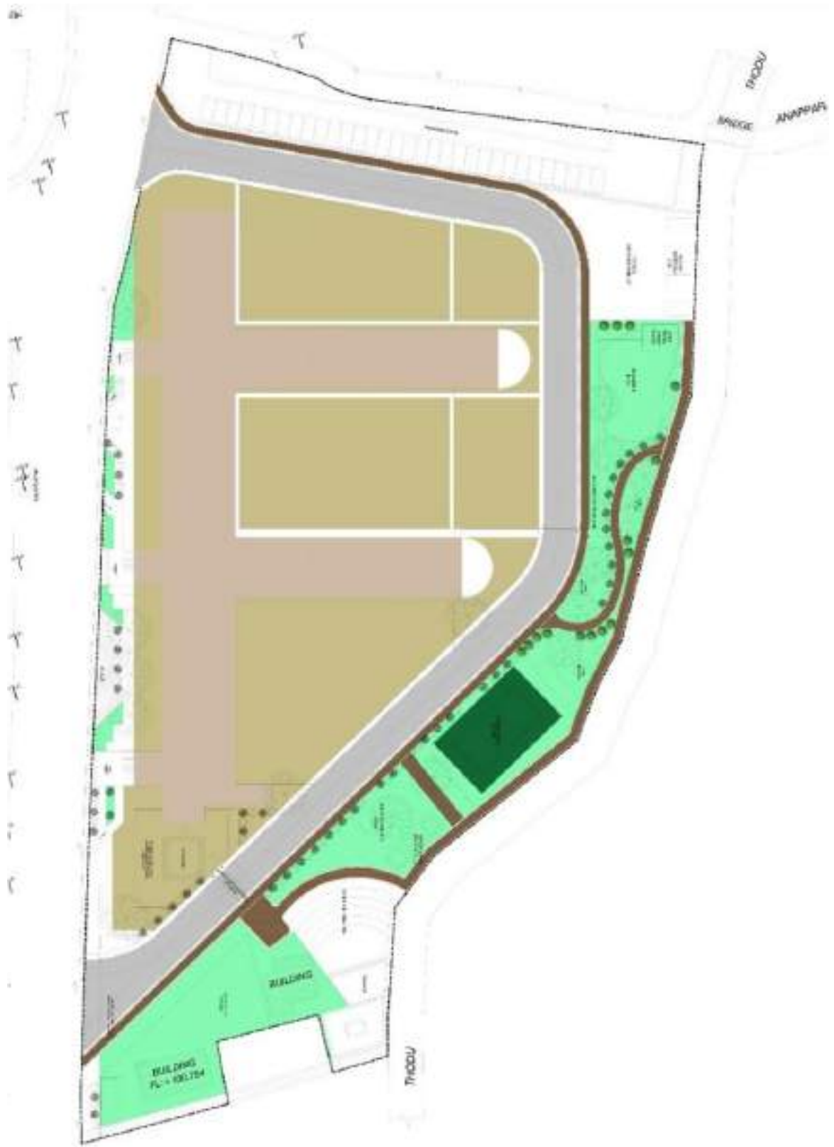
Figure 5-20: Proposed layout plan for Municipal Bus stand
